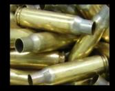
Ammunition Annealing ammunition casings 1-10 kW
