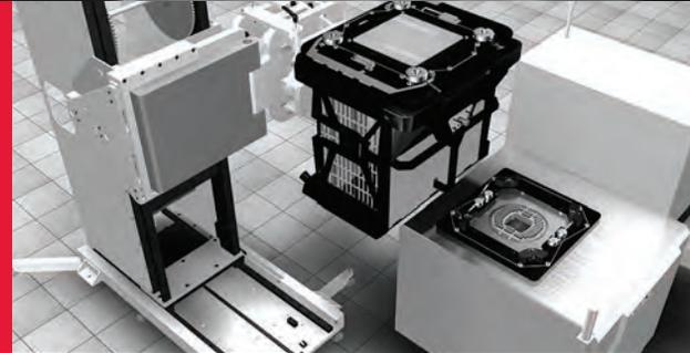
signals from the tester into the IC's circuitry. A returning signal leaves the IC and goes back to the tester for evaluation. Bad ICs are identified in this way and are discarded, so no further manufacturing effort—or cost—is invested in them.
